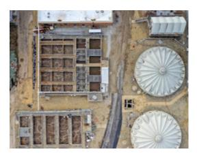
YBSD chose to upgrade the plant using Veolia's ZeeLung<sup>™</sup> MABR technology in combination with enhanced biological phosphorus removal (EBPR). The ZeeLung MABR is an energy-efficient solution that intensifies the treatment process while reducing energy consumption. It also reduces carbon emissions thanks to aeration energy savings, mitigation of nitrous oxide emissions and avoiding the construction of new concrete tanks.
