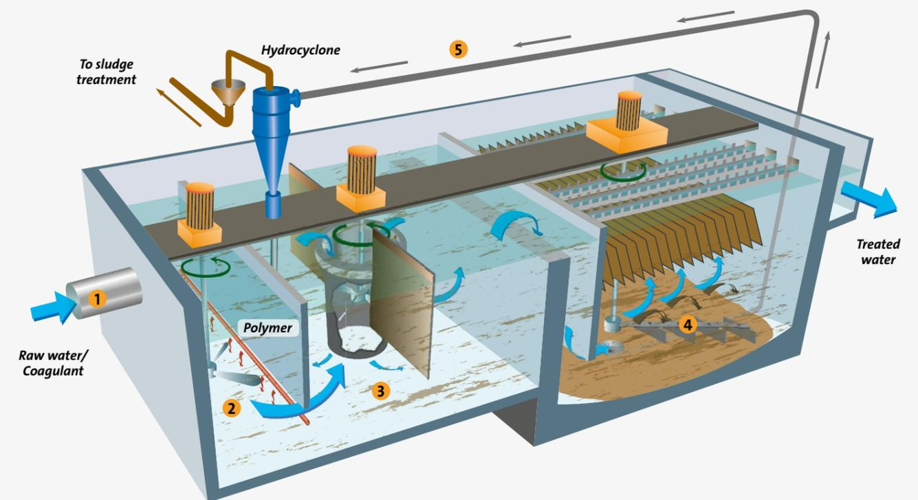
**1 Chemicals:** a coagulant, such as an iron or aluminium salt, is added to the raw water.
