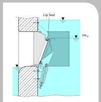
Figure 3: HYDROVEX® Flap Spring Loaded Weir with upper lip/seal for backflow prevention
