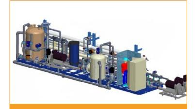
Hiprode, a totally new design in RO seawater desalination units. It allows optimum use of the greater permeability of the new membranes available on the market, thereby improving efficiency and reducing the size of the facility and its cost. The prototype tests conducted on this new configuration in a desalination plant operated by Veolia in Gibraltar were completed with success at the end of 2014, allowing the integration of this technological improvement in VWT's offering.
