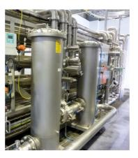
The customer expands the production facility in Cairo by a new water treatment line for carbonated soft drinks with a capacity of 200 m<sup>3</sup>/h. The main goal is to implement an efficient and sustainable water treatment solution by using the best available technologies in accordance with the international system design standards of the customer.
