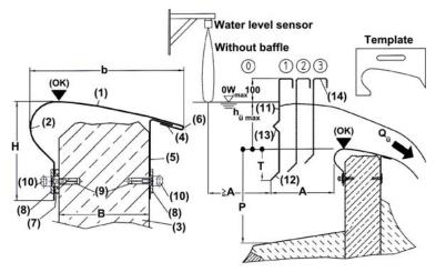
Figure 1: Hydrovex<sup>®</sup> FluidWing Installation
